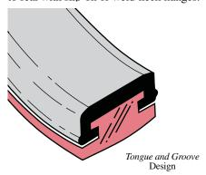
The seat features a molded O-ring which eliminates the use of flange gaskets. An important maintenance feature is that all resilient seats for Bray® butterfly valves Series 20, 21, 30, 31 and 34 are completely interchangeable.
