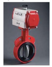
For severe corrosive applications the one-piece disc/stem and seat are offered in PTFE with a standard Nylon 11 coated body. The basic seat design is PTFE bonded to EPDM and incorporates a unique primary/secondary sealing design. This PTFE valve provides excellent internal and external corrosion protection. Refer to Bray Technical Bulletin and brochure on PTFE, Nylon 11, and elastomer-covered Series 20/21 for further details and design features.
