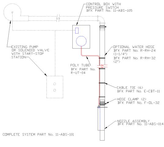
\*MOUNT CONTROL BOX AS CLOSE AS POSSIBLE TO THE WATER FILL HOSE/NOZZLE ASSEMBLY TO KEEP THE POLY HOSE SHORT.
