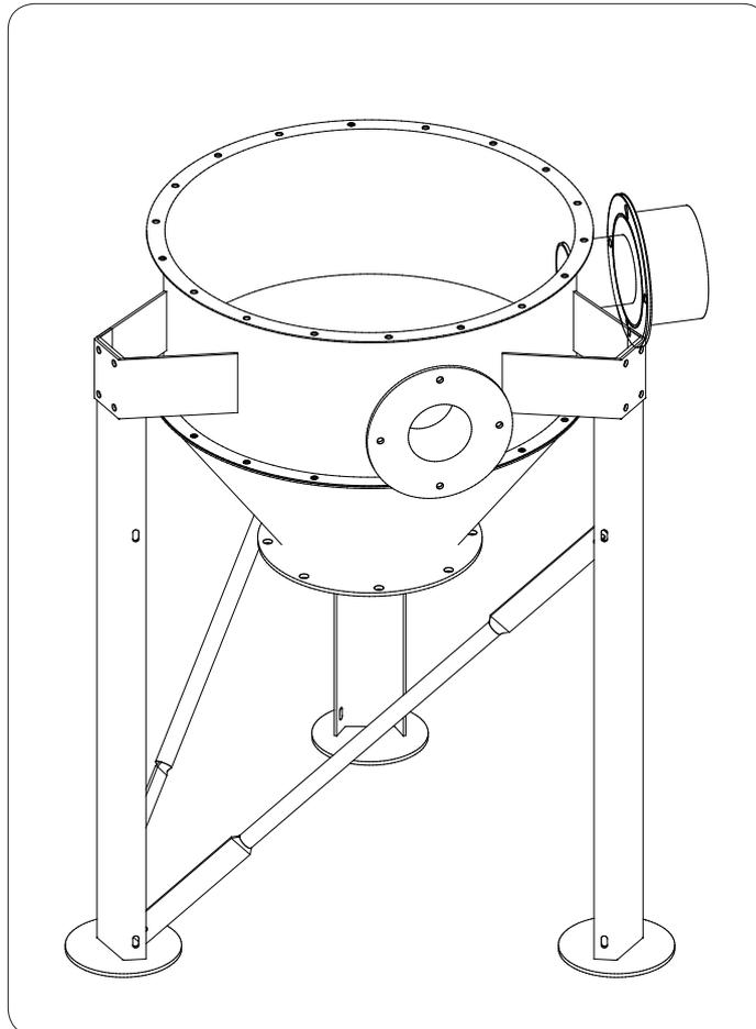
If it is found to be necessary to check the SILOTOP<sup>®</sup>R03 filter emissions (basic supply) a special kit is available for conveying all the air from the filter outlet into a single pipe.
