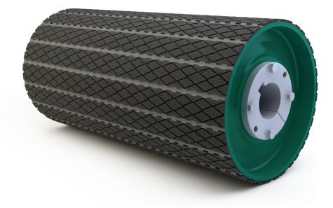
Craft-Lag<sup>®</sup> is designed to be a field replaceable lagging. It is bonded to a 5" wide rigid steel backing, which is then factory formed to a specific pulley diameter.
