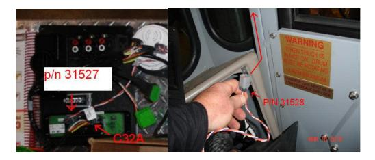
4) Cut the end off of the headlight switch connector and splice into the new harness with the splices that are already installed. Take care to ensure that the wire numbers match when splicing the wires and melt the heat shrink on the butt connectors when finished. Plug the headlight switch connector on the new harness (C34) into the headlight switch.
