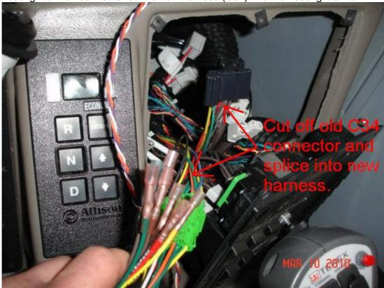
5) Run 94" jumper harness (p/n 31528) up cab upright to the new slump gauge in the overhead console and plug in.
