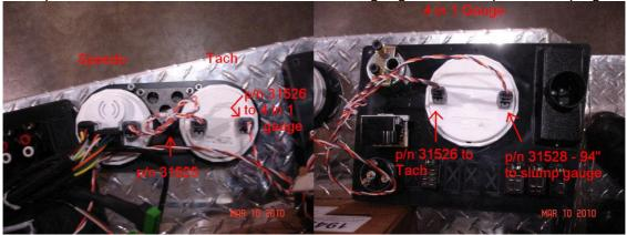
7) Plug jumper harness from the slump gauge (**p/n 31528**) into the other port in the 4 in 1 gauge.
