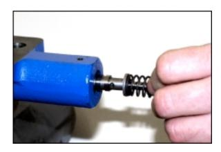
Use a 1/8 hex head wrench to remove the shoulder screw, spring retainer, spring and spring box spacer. Discard spring and shoulder screw. We are now ready to reassemble the control with the new components.
