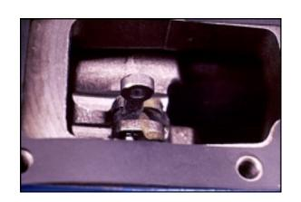
Lubricate and install the new dust seal over the shaft with the lip of the seal facing upward. Using a deep-wall socket or similar tool, carefully press or drive the seal in until it contacts the bottom of the counterbore in the control housing.
