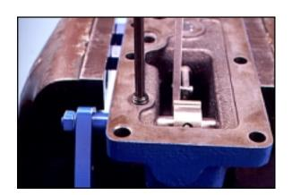
With the shaft set screw backed out, slide the shaft assembly over to disengage the link from the control spool. Next, pull the link assembly upward past the spool and slide it over to disengage it from the connector.
