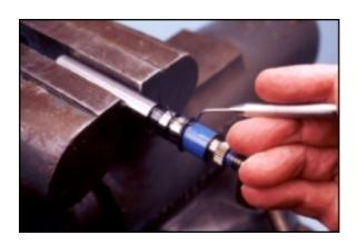
**Step 10**Lubricate the sealing ring and install in groove located in the shaft.
