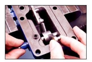
Assemble the small connector link to the new, longer link assembly. When assembling the two links, the pins must face the same direction. After assembly, install the new small retaining ring.
