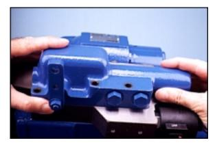
**Step 25**Install the new retaining cap screws. Torque cap screws to 16 ft. lbs. [22 Nm].
