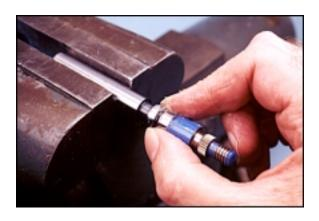
**Step 11**With the previously started connector pin pointing toward the spool, install control shaft into housing and connector/link assembly.
