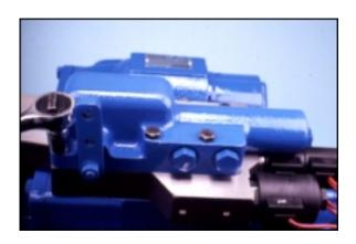
`990815-000 (replaces 990787-XXX) without Manual Displacement Control configured with 1, 2-pin connector and 1, 4-pin connector (not shown)
