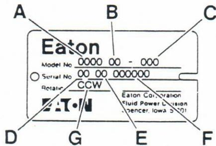
A — Displacement ( cu. in. / rev. )
