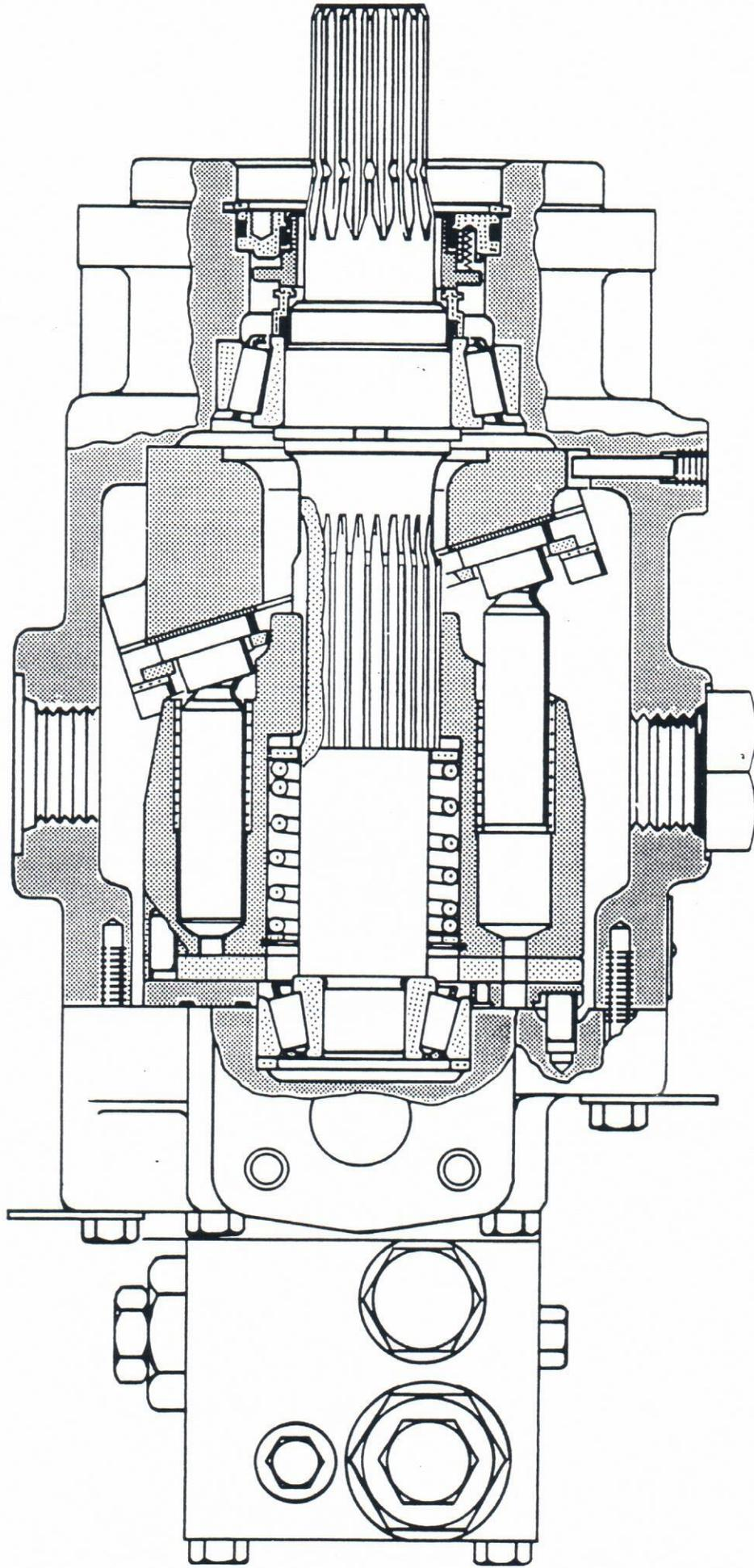
Hydrostatic Motors Series 1 – Fixed, Models 33 thru 64
