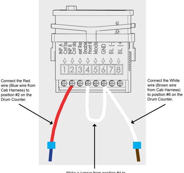
Make a jumper from position #4 to position #6 on the Drum Counter.
