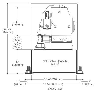
Nominal Dimensions are shown for all basic components. Dimensions may be found for your particular system by deleting the component shown on the unit drawing and adding the dimension for the same item you have selected. Note: Dimensions may vary slightly and should be confirmed by the factory if unit is to be installed in space with minimum clearance.
