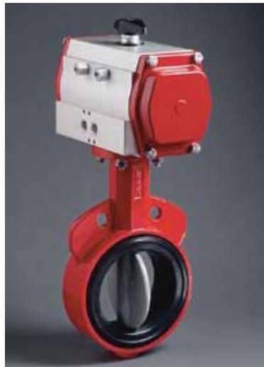
For severe corrosive applications the one-piece disc/stem and seat are offered in PTFE with a standard Nylon 11 coated body. The basic seat design is PTFE bonded to EPDM and incorporates a unique primary/secondary sealing design. This PTFE valve provides excellent internal and external corrosion protection. Refer to Bray Technical Bulletin and brochure on PTFE, Nylon 11, and elastomer-covered Series 20/21 for further details and design features.
