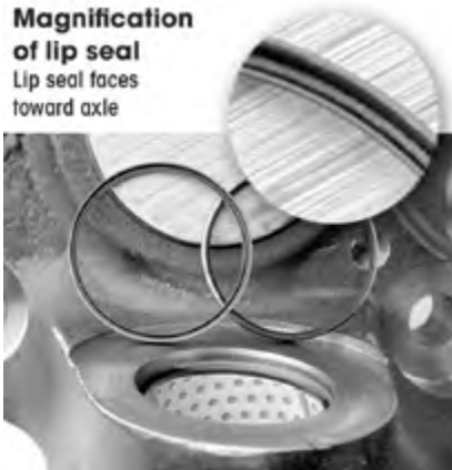
FIGURE 10 STEERTEK NXT Magnification of the kingpin bushing and a DOUBLE lip seal installed in the steering knuckle.
